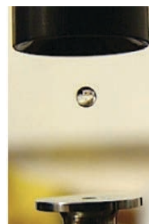
Figure 1: Images of a \alpha -pinene droplet levitated in an ultrasonic trap.
